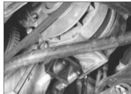
12.4 Remove the pivot bolt and nut
